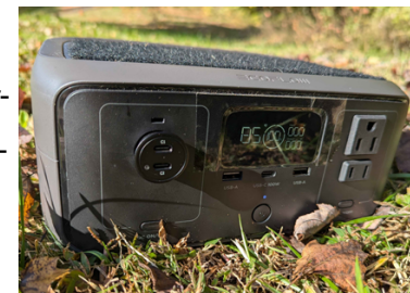
Modern Portable Power Stations are now a feasible option for running radios in the field, if users are aware of their limitations and potential EMCON concerns.
